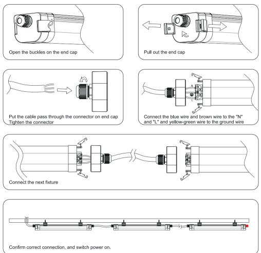
Wiring (two cables from single end)
